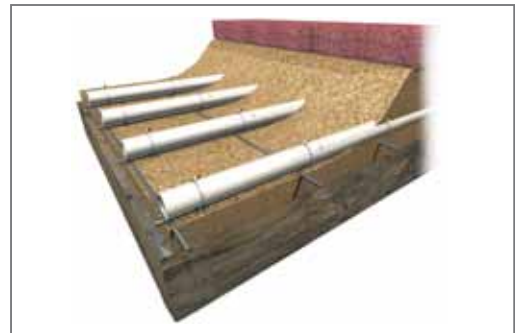
Floor heating in open spaces
