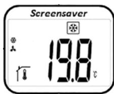
From this screen, pressing the  $-$  or  $+$  key will show the set target temperature (flashing). By pressing the  $-$  or  $+$  key, the desired target temperature can be set. By pressing the  $OK$  key, the desired target temperature is confirmed.
