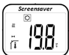
From this screen, pressing the  $-$  or  $+$  keys will indicate the pre-set target temperature (flashing). Pressing the  $-$  or  $+$  keys again will set the desired target temperature. By pressing the  $\text{OK Mode}$  key, the desired target temperature is confirmed.
