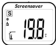
From this screen, by pressing the  $-$  or  $+$  key will indicate the pre-set no. of revolutions (flashing). By pressing the  $-$  or  $+$  key again, the desired no. of revolutions can be set.
