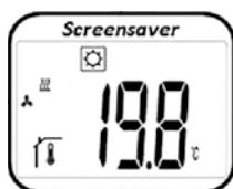
From this screen, pressing the or keys will show the pre-set target temperature (flashing). Pressing the or again will set the desired target temperature. By pressing the Key, the desired target temperature is confirmed.
