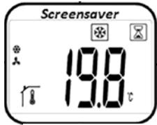
From this screen, pressing the  $-$  or  $+$  keys will show the set target temperature (flashing). By pressing the  $-$  or  $+$  keys you can set the desired target temperature. By pressing the  $OK$  key, the desired target temperature is confirmed.
