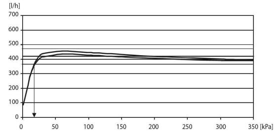
Schematic view of the flow characteristics of the insert with a nominal flow of 420l/h. The insert limits the flow to a minimum of 21 kpa and keeps it up to a maximum of 350 kpa before overflow is obtained.
