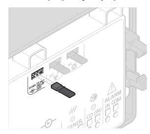
This jumper is for setting the delay time (no delay or 5 minutes delay) of the Boiler/heat pump control output to turn Off after the last thermostat stop sending demand for heat (or cool).
