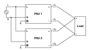
Fig. 4 Parallel Operation Connection Diagram
