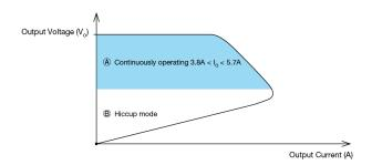
Additionally, if the  $I_{\rm O}$  is >102~108% for a prolong period of time (depending on the load), the Over Temperature Protection (OTP) will be activated due to high temperature on critical components. The power supply will then go into "Latch mode" until the PSU cools down and the AC power is recycled.
