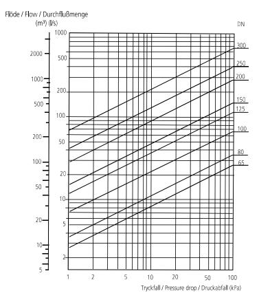
We recommend a pressure drop of 5-10 kPa for dimensioned valves.
