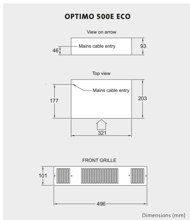
**N.B:** Add 4.5mm to the chassis height to allow for rubber mountings and screws.
