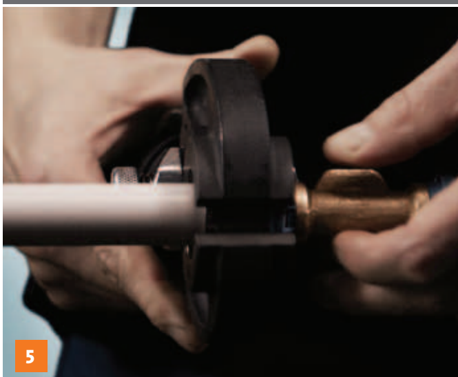
Adjusting the fitting to TH conthur jaw
